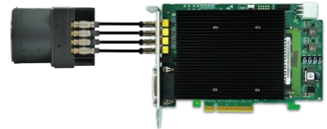
Figure 29 – Single camera topology
