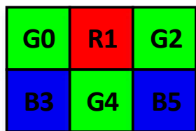
Figure 15 – Bilinear de-mosaicking algorithm (Line scan)
